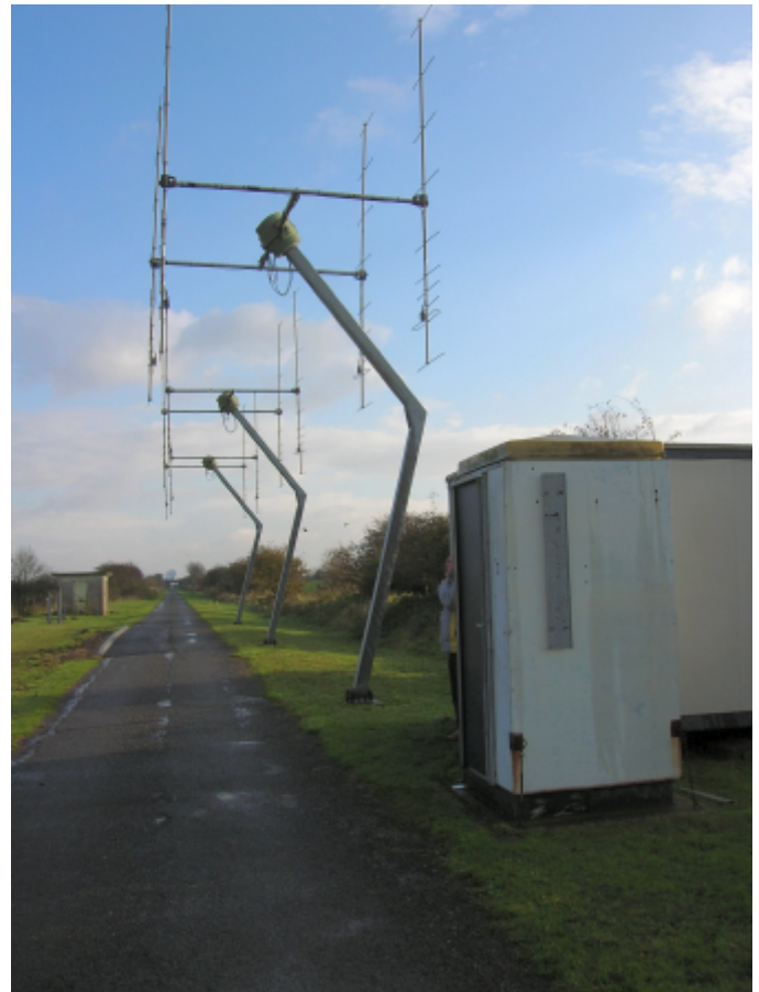
Three of the four Yagi arrays and the BAA Hut, at the MRAO
