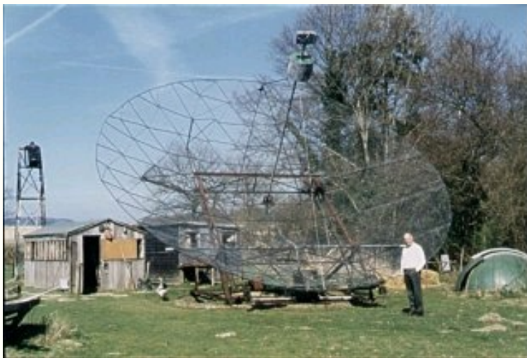
Left: John Smith with his home made 9m dia.parabolic antenna
