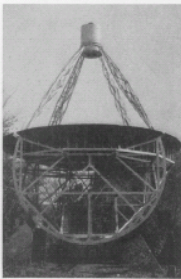
Fig. 1—Antenna system used for the investigation of cosmic static.
