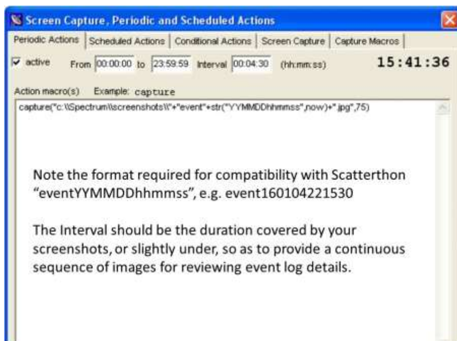
Fig 3 Using the Periodic Actions function to take a complete set of screenshots for subsequent verification of the event log details
