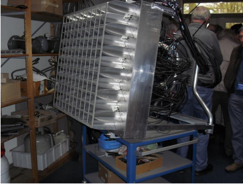
(Figure 7 An APERTIF FPA unit with its 121 Vivaldi antennas.)
