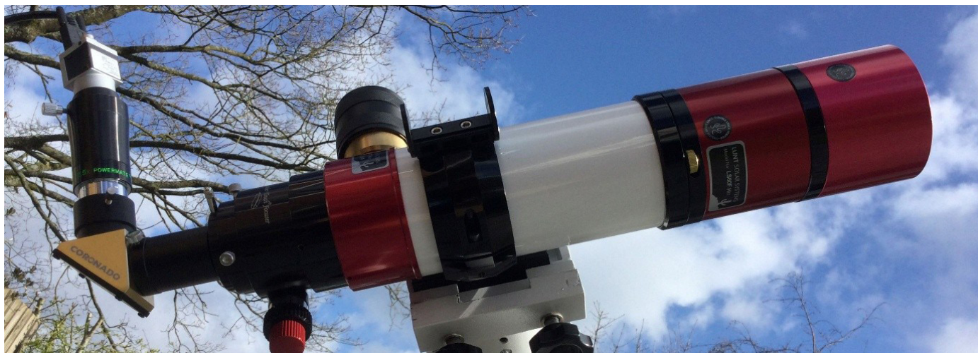
Stuart's Lunt 60 solar telescope fitted with additional filters to create a triple stacked narrowband scope to capture full disk images of the Sun at 656.28 nm.
