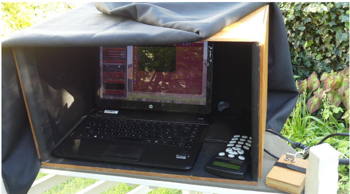
Figure 12. The writer's computer box set up for imaging Mercury, with the dark cloth folded back. The telescope drive controller is inside the box beside the laptop, and the focuser control is next to the box on the right.
