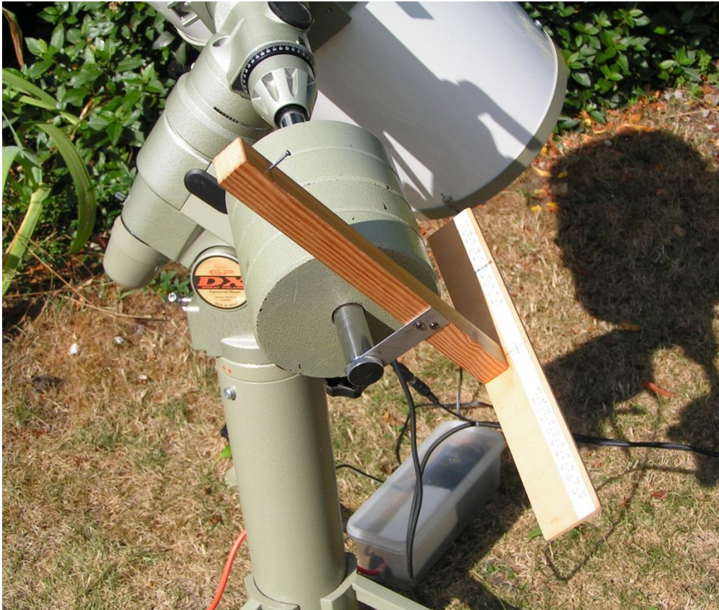
Figure 5. The writer's GP-DX mount showing the device used for offsetting in RA to locate Mercury. The telescope has been moved west so the shadow of the nail falls on the calculated point.
