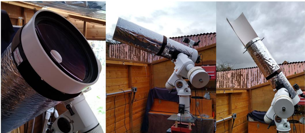
Figure 3. Example of a light-baffle. Chris Dole's 180 mm Maksutov (left panel) with the normal dew-shield/light baffle (middle panel) and the temporary extended light-baffle (right-hand panel).
