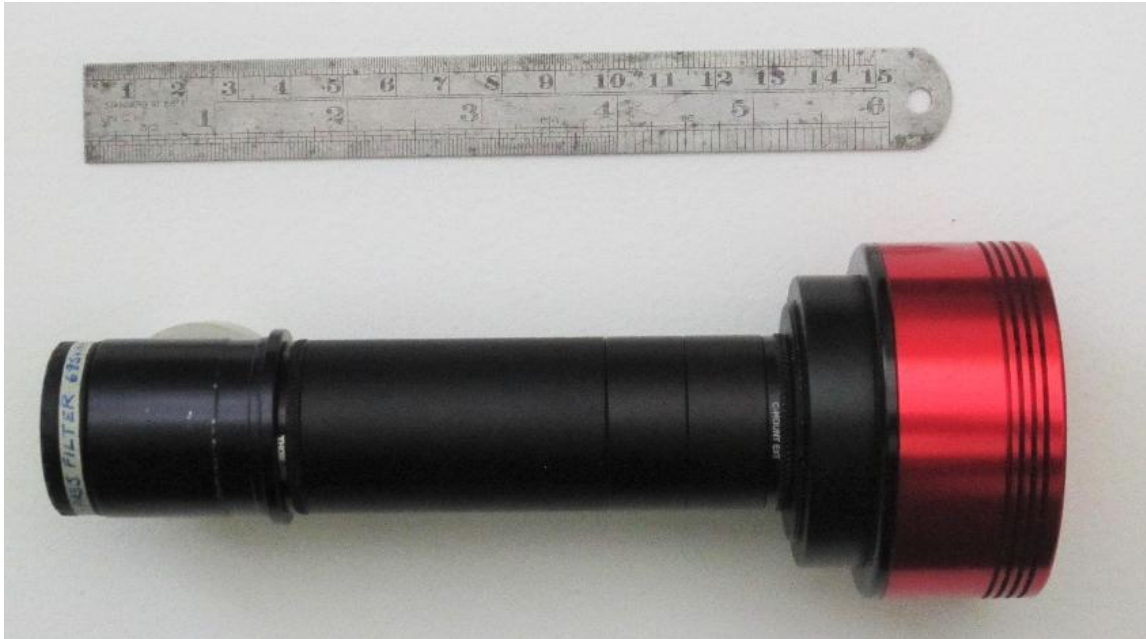
Figure A1.2. The assembled IR Barlow lens attached to the ASI174MM camera ready for use.
