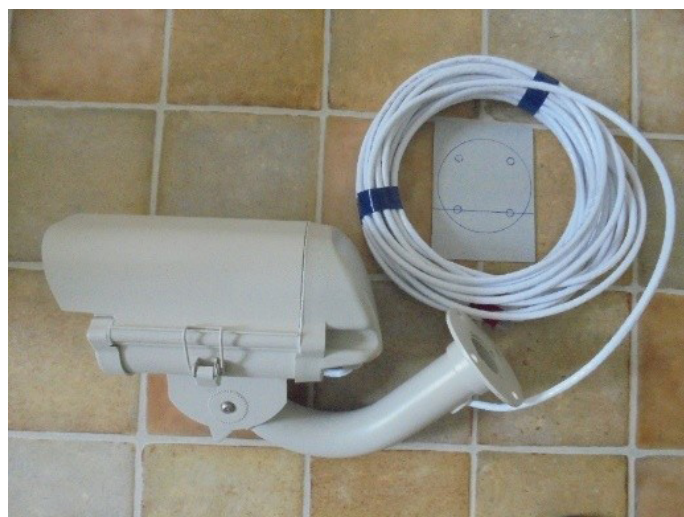
Image of camera housing including the drilling template
