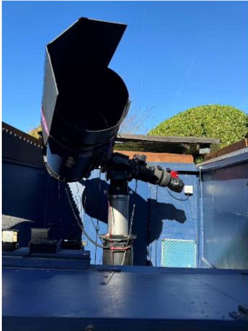
Figure 4.4. Using a suitable lightweight shield with a 14inch SCT when Venus is close to the Sun, to protect the imaging chain from direct sunlight. (Peter Tickner)
