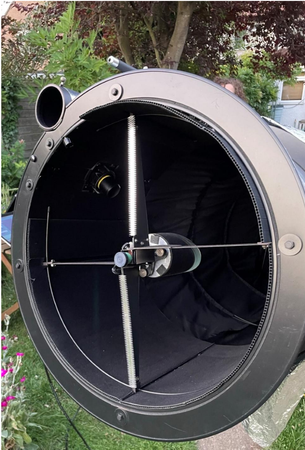
Figure 5.18. Apodising mask consisting of a 30° saw-tooth on 3mm pitch and attached to the two offending vanes of a 444mm scope.
