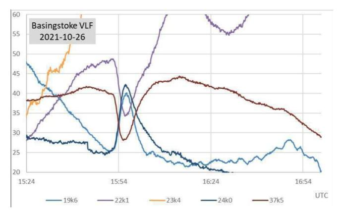
This recording from Paul Hyde shows the M1.0 flare peaking at 15:56UT on the 26<sup>th</sup>. The 23.4kHz signal is rising steeply into the sunset, but the other signals all show good clean SIDs.
