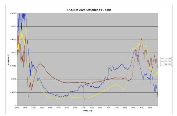
This magnetic activity was also recorded on the 37.5kHz signal by Mark Edwards. The chart shows the 12<sup>th</sup> in blue, with the 11<sup>th</sup> and 13<sup>th</sup> in brown and yellow. There appears to be a signal drop-out just after 13:00 on the 12<sup>th</sup>, but the rest of the day is clearly very disturbed. Colin Clements also recorded a similar disturbance at 37.5kHz, matching well with Mark's timings.
