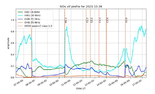
Mark Prescott has added the peak timings for each of the flares to his recording. This helps to identify the 'peak and wave' SID from the M2.2 flare, as well as the unusual 20.9kHz SID from the X1.0 flare.
