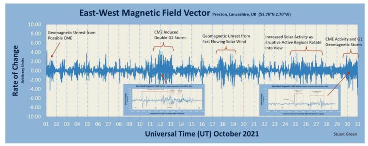
Stuart's chart for October shows that it was a very active month, with a number of CMEs as well as fast solar winds. The period around the equinoxes always show a greater influence from the inter-planetary magnetic field, due to the more favourable alignment with the Earth's field at this time of year.
