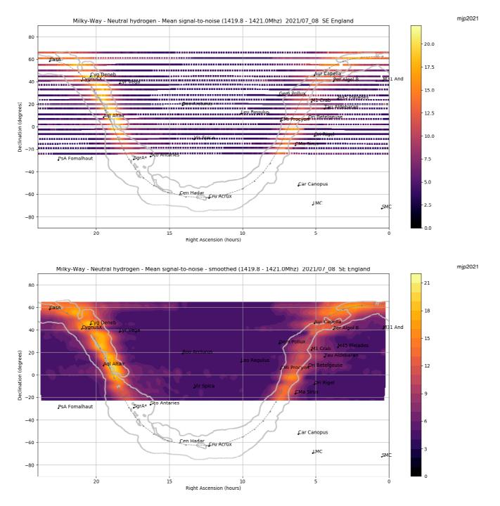
The first chart shows the data from the individual drift scans, overlaid onto a map of the Milky Way. The second chart shows the smoothed data signal-to-noise ratio over the area observed. The strongest signals follow the known position of the galactic arms extremely well. The data was also used to calculate the galactic rotation curve, with results closely matching those derived from the ESA GAIA survey data.
