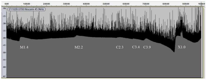
Colin Briden recorded the 45.9kHz signal from Niscemi, Italy, SIDs showing in the grey area, black indicating the raw signal data. Here all of the flares have produced ordinary 'shark fin' SIDs.
