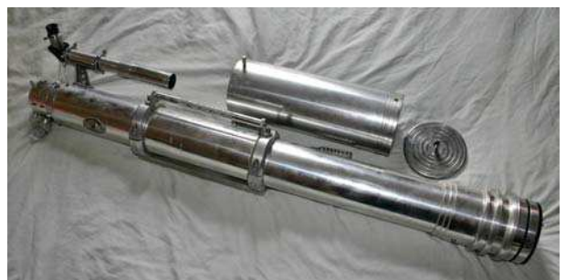
The 100-mm f/13 Moonraker refractor by Turner.
