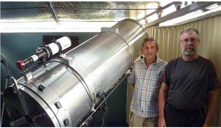
Figure 3. The 508mm f/4 Newtonian reflector of Phil Miles (left) with Anthony Wesley (Rubyvale, Queensland, Australia).
